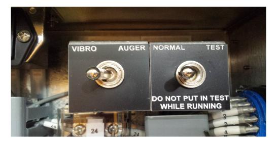
This bulletin is to address the possible danger of the engine not being able to be shut off because of the **NORMAL/TEST** switch in the panel. If you select the test option while the engine is running there is no way to shut the engine off safely. The switch will have to be put back in the normal position to be able to use the **OFF** and **E-STOP** selections.
