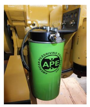
This is the auxiliary engine oil filter kit (1001427) we use in our power units. This unit filters 1 guart per minute at one micron. The inlet is being supplied from the same port as the engine oil pressure gauge. The return oil is set back to a different location on the engine block depending on model.
