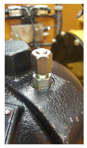
Below is the part number for the KIT that replaces the bleeder in the pressure filters. The fitting is a SAE to JIC fitting with JIC cap.
