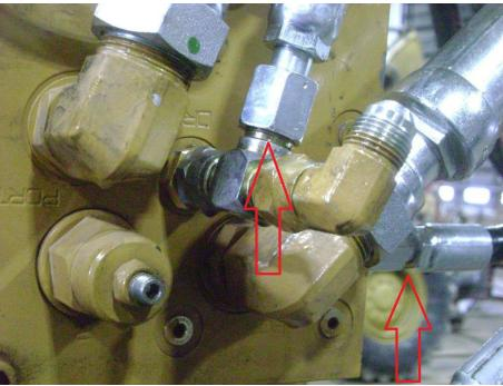
Here is a tee installed to the case drain port so that the shuttle valve can be externally connected to the case drain circuit. The arrows show the hose ends connected to the shuttle valve and the case drain tee.
