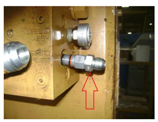
Here is a picture of the external ported shuttle valve. The fitting is screwed into the end. This valve sends the oil out of the fitting instead of through the manifold.
