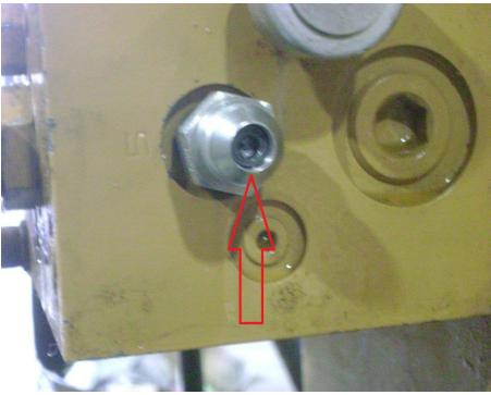
In this photo you can see the orifice installed.
