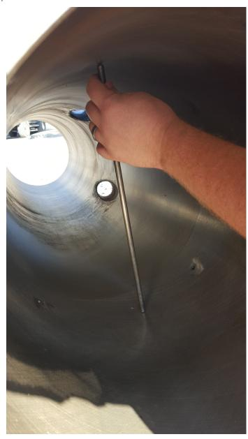
Using a Go/No-Go gauge, you can quickly check the cylinder tolerance. When using this gauge it is extremely important that you are sweeping in the center to get an accurate measurement.
