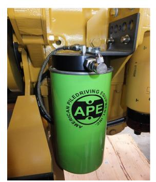
This is the auxiliary engine oil filter kit (1001427) we use in our power units. This unit filters 1 quart per minute at one micron. The inlet is being supplied from the same port as the engine oil pressure gauge. The return oil is set back to a different location on the engine block depending on model.
