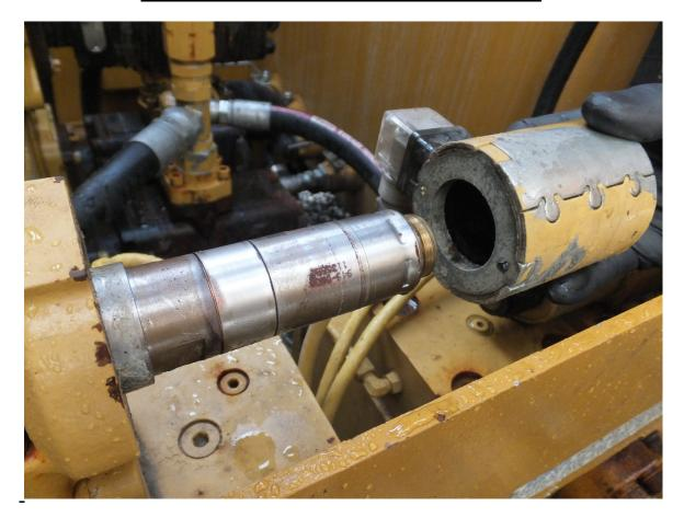
This bulletin is to help with the servicing of our control valve solenoids. When conducting a servicing of the filters, these should be serviced also. In this picture you can see surface rust; the rust will need to be removed with emery cloth or abrasive pad.
