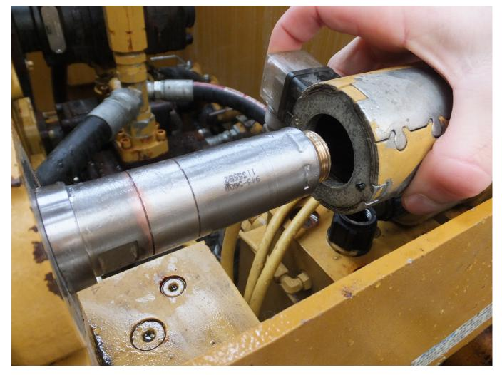
Here is a picture after being cleaned, and die electric grease added ready for install. The electrical DIN connector should be on the side, not the top; this will assist with water to drain from the connectors.
