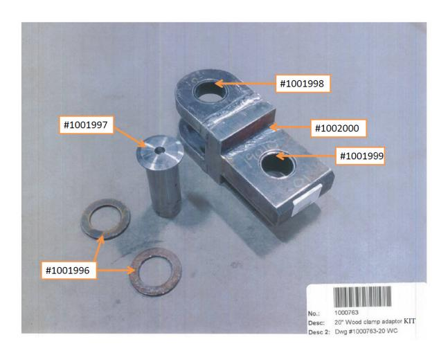
This is a wood clamp extension used to remove or reduce the amount of plate spacers on the fixed jaws of our 20", 25", and 32" wood clamps. We are currently inventorying these kits and individual components in the parts warehouse.
