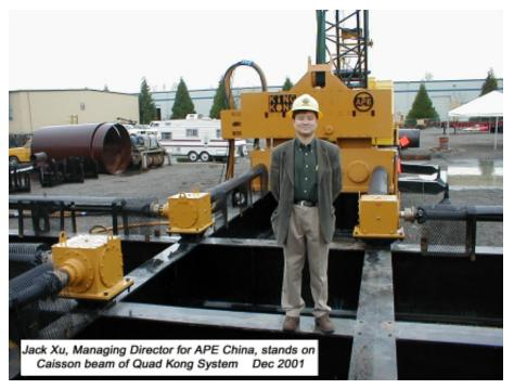
Jack Xu stands next to the four Model 400 vibros mounted on a test caisson beam at the APE testing facility in Kent,
