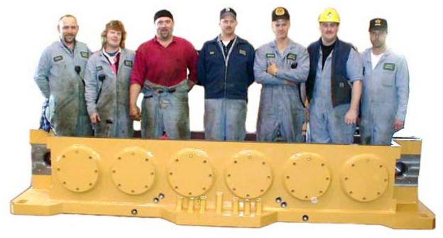
The APE Model 600 is a larger version of the APE Model 400. The 600 has 20,000 inch pounds of eccentric moment. The design is a stretch version of the Model 400. It has six counterweights.
