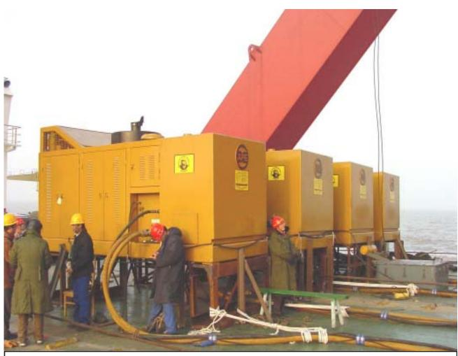
Four APE Model 1000 power units teamed together to provide 4000 horsepower to drive the APE Model 400 Quad Vibratory driver/extractor. Four CAT 3412E electronically controlled engines are fitted to a special control system.
