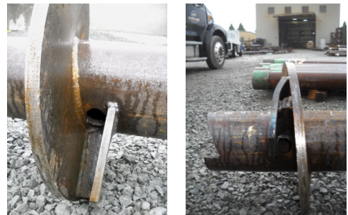
Photo B-1. Pile 2 grout hole.
