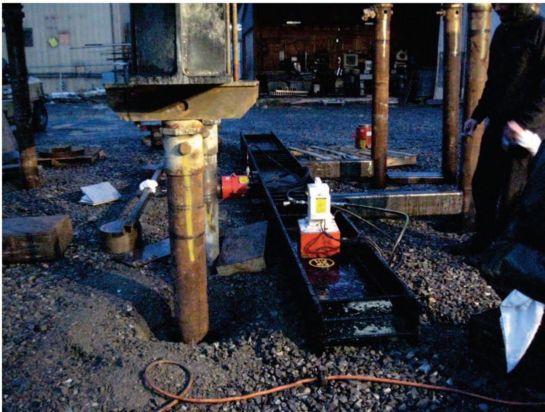
FIGURE C-3 Lateral Load Frame Photo
