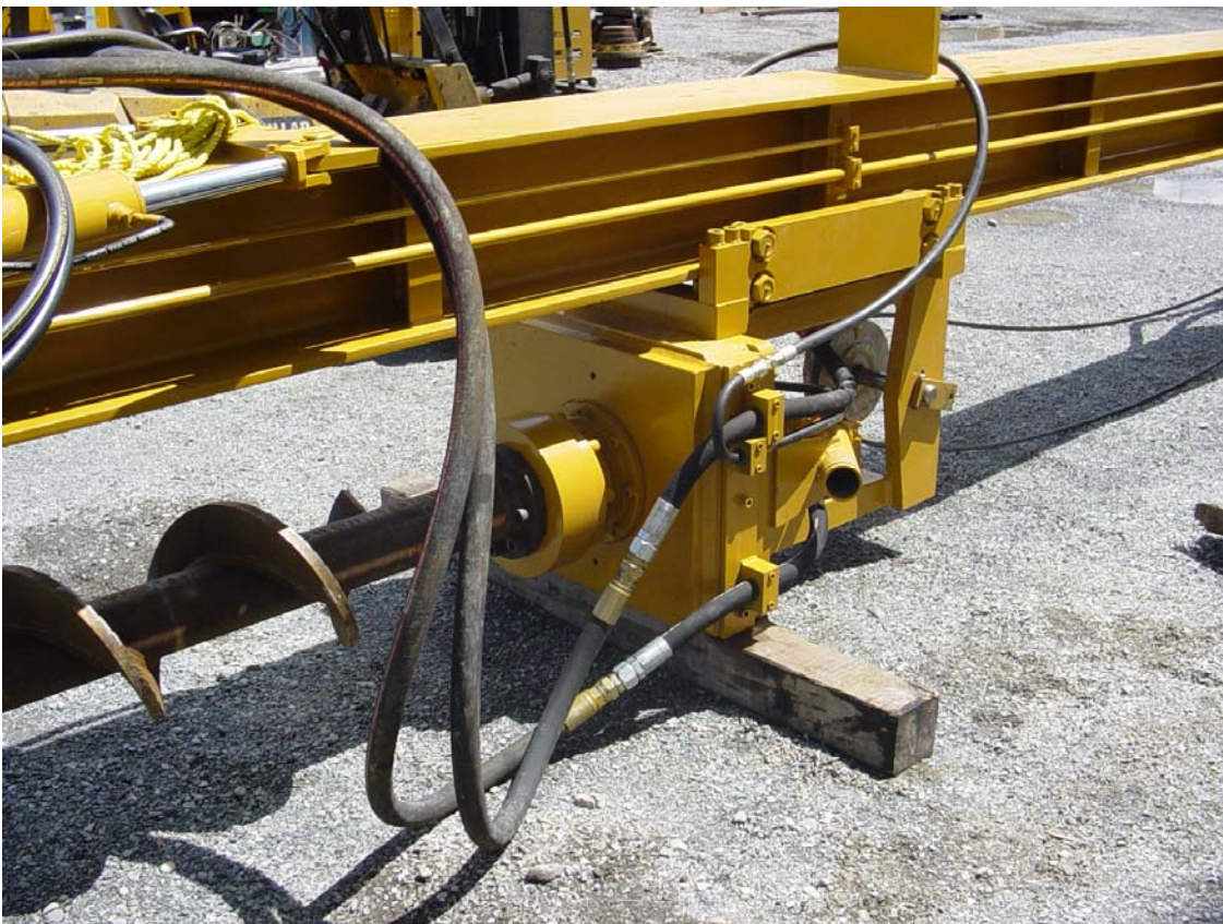
PHOTO 2: DRILL MAST ASSEMBLY WITH 3060 DRILL
