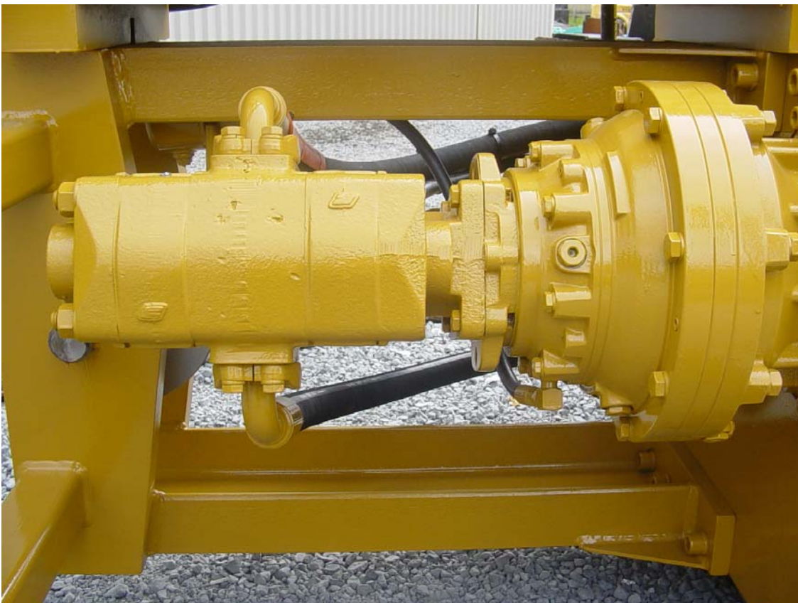
PHOTO 28: DRILL MOTOR HOOKUP
