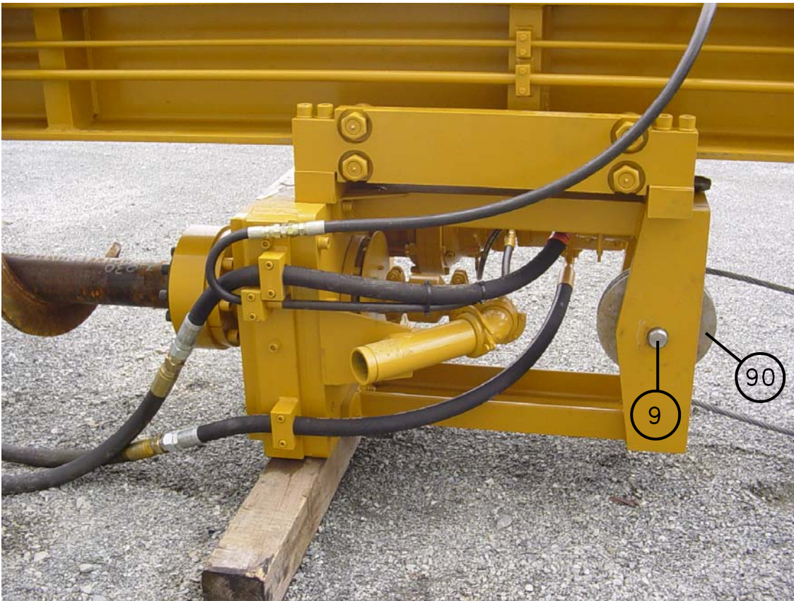
PHOTO 27: 3060 DRILL SHOWING PIGTAILS
