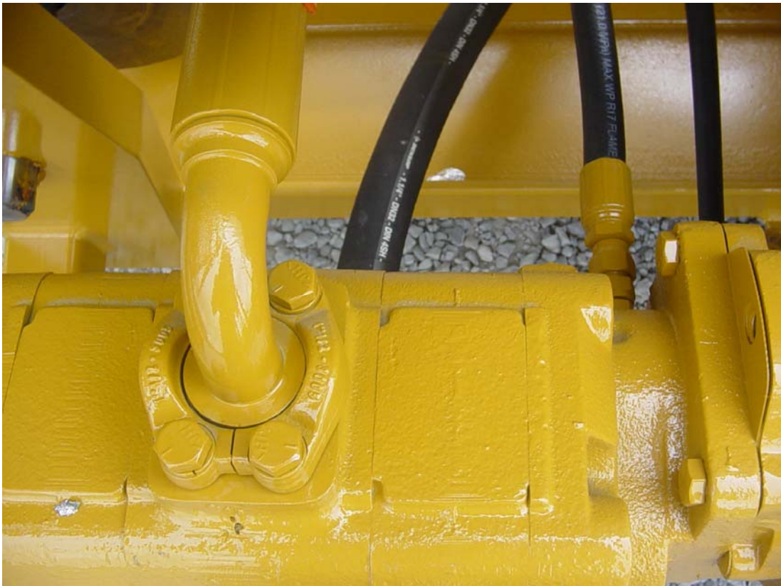
PHOTO 30: DRILL MOTOR HOOKUP
