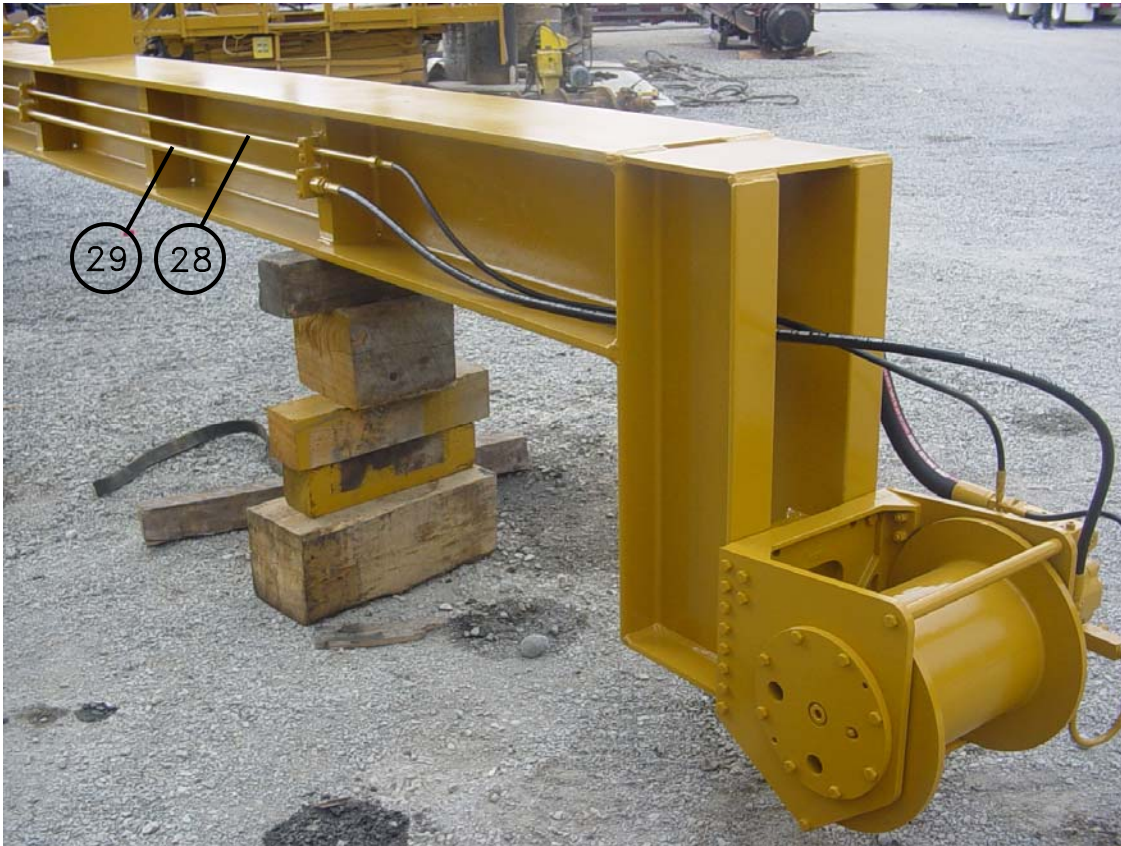
PHOTO 23: TOP WINCH – DRAIN & SIGNAL
