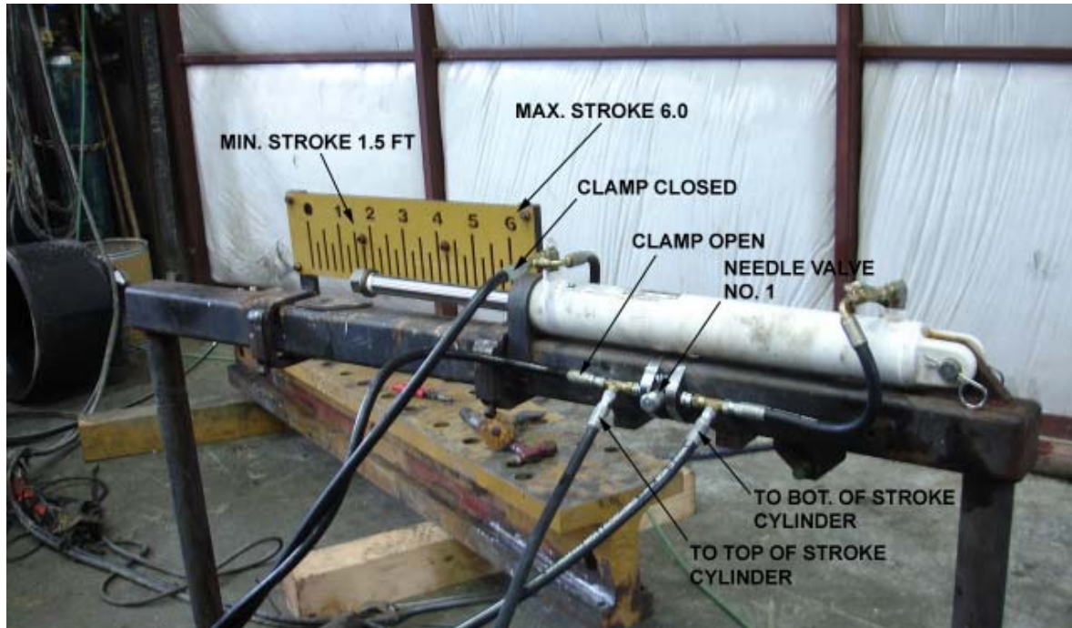
Figure 2G. Visual Stroke Indicator Cylinder
