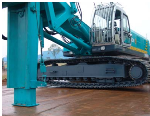
Fig. 8 Crawlers extend and retract
